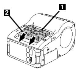
4. Wipe off any dirt on the platen and peel roller (1) using a cloth soaked in alcohol.
